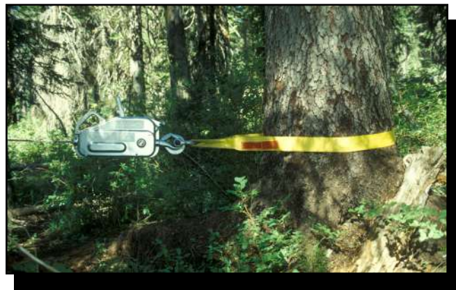
Figure 5—Grip hoists are used to tighten rigging cables.
